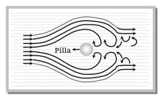
energy maintaining the flow is spent in producing eddies in the liquid and only a small fraction of energy is available for forward flow. For example, eddies are seen by the sides of the pillars of a river bridge.
