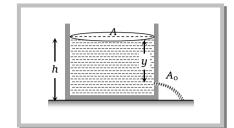
If the hole is at the bottom of the tank, time *t* taken to make the tank empty:
