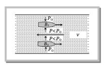
(ii) Working of an aeroplane: This is also based on Bernoulli's principle. The wings of the aeroplane are of the shape as shown in fig. Due to this specific shape of wings when the aeroplane runs, air passes at higher  $\frac{v \text{ large, } P}{v \text{ large, } P}$
