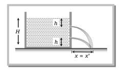
(v) If the level of free surface in a container is at height H from the base and there are two holes at depth h and y below the free surface, then
